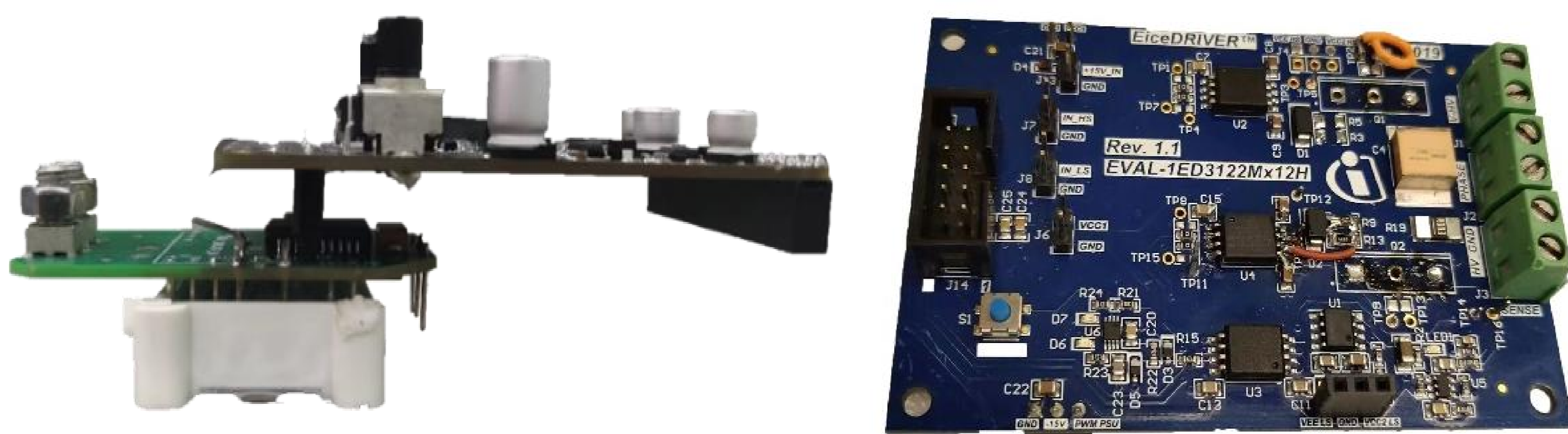
Fig. 6. Driver Board(Left), Infineon evaluation board (Right)
